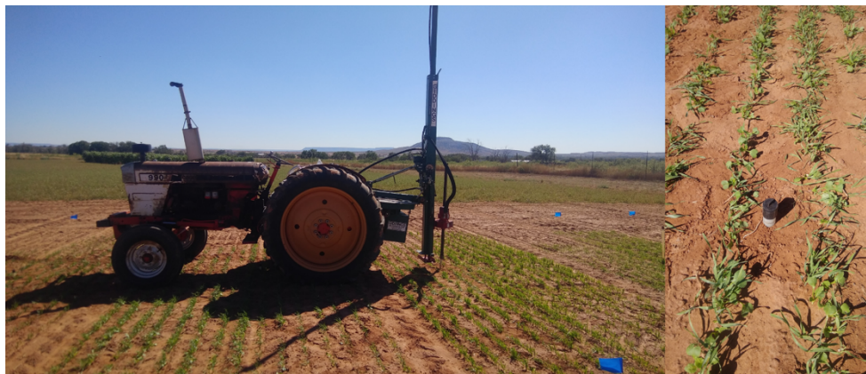
Installation of soil moisture measurement tubes after cover crop emergence.
